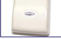
Repeaters automatically form the backbone mesh radio network, relaying messages to/from the Hub. The network physical layout is determined by the placing of Repeaters, which may extend across floors and buildings. Repeaters are battery powered and do not need any wires, making installation very quick and low cost. Each Repeater provides a location beacon signal for accurate location determination for alarm signals and also for tracking.
