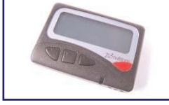
The Pager is multi-function supporting display of received messages with acknowledgement plus the ability to generate an alarm from the User, Dead-Man or Man-down Features. The Pager displays shows alarms from other Pagers and Call Fobs, allowing the User to accept the alarm and signal back to the Call Fob or Pager User sending the alarm that assistance is on its way.
