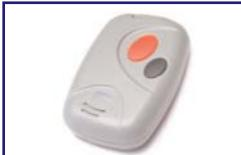
The Call Fob allows an assistance call to be generated either by the User pressing a button or automatically by the Dead-Man or Man-Down features. Accurate location information is obtained from nearby Repeaters. The Call Fob can also report the User's location to a Hub web page as the User moves around, allowing User tracking applications such as patient or visitor location to be implemented. Acceptance of assistance calls by an EkoTek Pager is indicated at the Call Fob to reassure the User.
